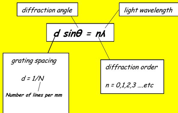
**USE OF DIFFRACTION GRATING TO MEASURE LIGHT WAVELENGTH**
