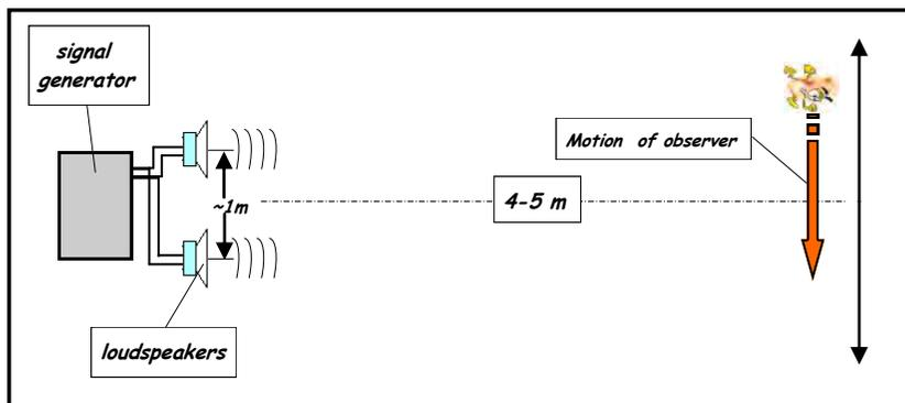
Two loudspeakers are connected to a single signal generator as shown in the diagram. The sound waves emitted by each speaker are then of equal frequency, wavelength and amplitude. An interference effect due to the superposition of the sound waves is observed in the region in front of the speakers.
