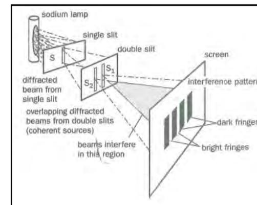
The sodium lamp acts as a monochromatic (single wavelength) light source and it illuminates the narrow slit (**S**). Diffraction at **S** causes a diverging beam of light to fall on the two narrow slits **S<sub>1</sub>** and **S<sub>2</sub>** which are very close together and parallel to **S**. Since they are derived from a single source **S**, the two slits act as **coherent** light sources.
