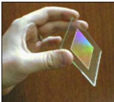
When a beam of monochromatic light is directed at a diffraction grating, it passes through the clear spaces between the lines and it is transmitted in certain, clearly defined directions only. This is because as they pass through the slits, the light waves are diffracted and those from adjacent slits interfere **constructively** in certain directions (maximas) and **destructively** in others (minimas).
